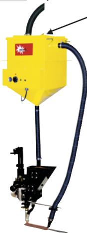
**Optional HFH-100** heated hopper (250 °F, 121°C) automatically gravity feeds recovered flux to lower welding system hopper. System available with magnetic separator, unheated and in different flux capacities (i.e. 200 lbs, 300 lbs, 600 lbs, 1000 lbs etc. ). Must be used with Mighty-Mac vacuum.
