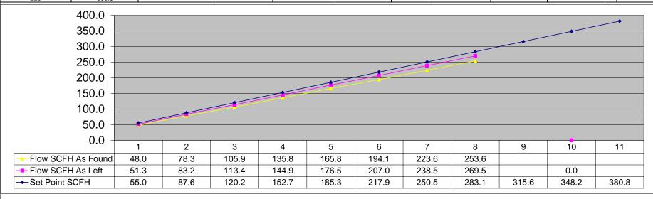
Changed the #56 orifice due to failure outside 5%.
